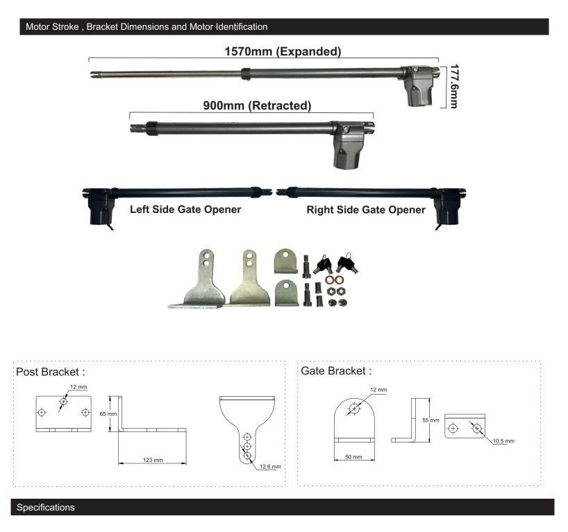
Motor Voltage Manual override Working temperature Maximum stroke Gates size Gate weight Absorbed power Current Motor speed Thrust 24v DC Via override key supplied -10° ~50° 650mm 3m max (for each gate) 175kg max (for each gate) 70W 5.2A 1800RPM 1800N Before beginning the installation of the gate motors a physical gate stop must be installed at the closed position.
