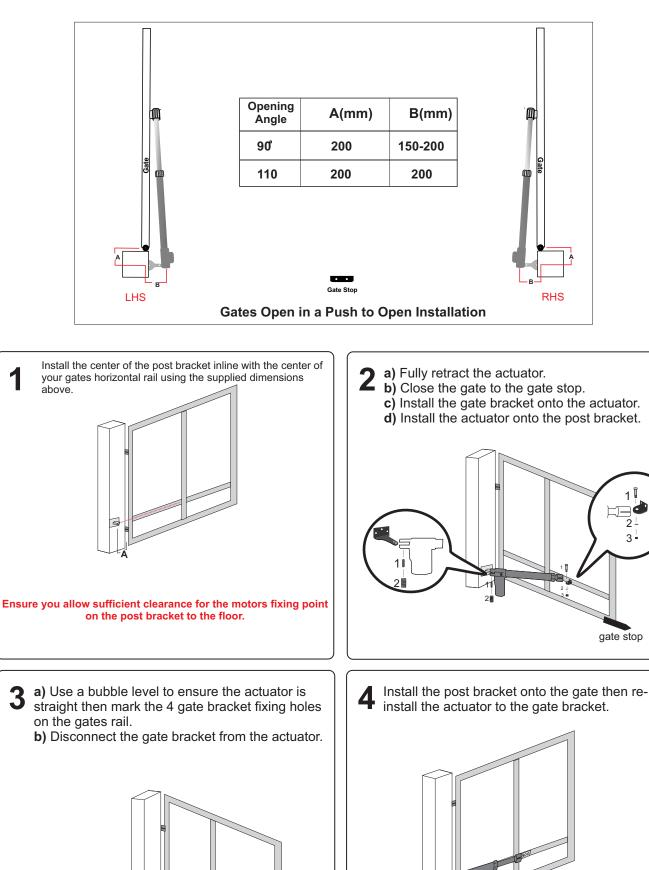
Motor installation complete Repeat steps 1 to 4 for second gate if applicable
